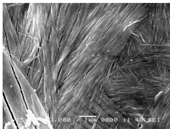
Fig. 1. SEM micrographs of polycinnamamide thorium (IV) phosphate (magnification, 13,000×).
